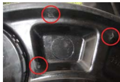
Impact is easily absorbed with no structural breakdown
