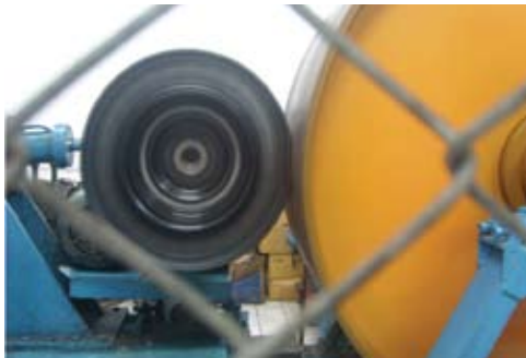
Tyron ATR undergoing load and speed testing
