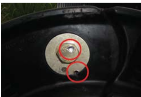
Minimum impact damage to runflat fixings
