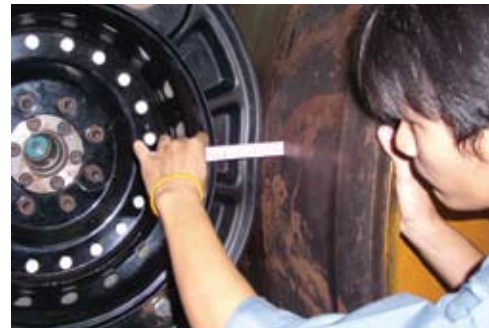
Measuring unique load deflection characteristics
